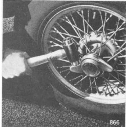
**Fig. i8.** Removing L.H. front hub cap.
