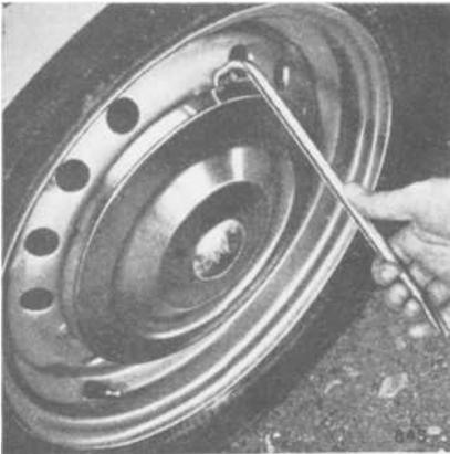
**Fig. 17.** Removing nave plate.
