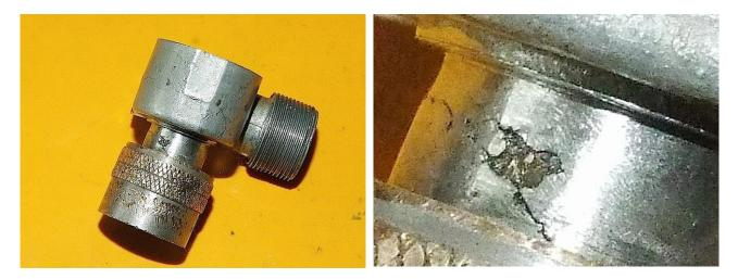
Here is another that has suffered abuse to its stem. In this case it has come undone from the transmission and has been running loose and rubbing on something. Again you can see how thin these are:
