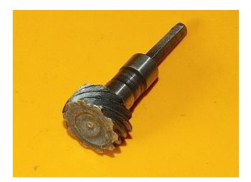
The gear-teeth get worse on the drives from the far-east. The teeth on this one have not been machine cut, they are just as they left the mould, when this item was cast. This one has had the ferrule knocked out also, you can see that there was no weld-penetration, just a suface mark where the weld was "stuck-on".
