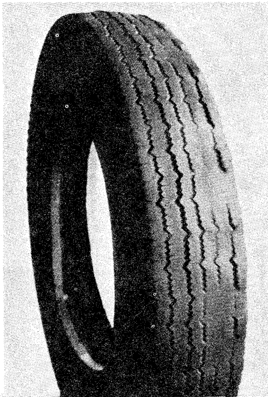
Fig. 11 “Spotty” Wear due to a variety of causes.
