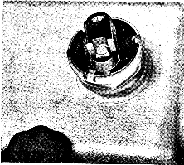
Fig. 38 Showing the position of the Isolator Switch on the Gearbox Cover.
