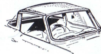
The 'Surrey Top' (a folding canopy of p.v.c.) quickly clips into position for emergency weather protection.
