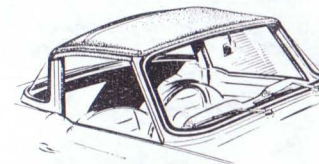
The 'Surrey Top' (a folding canopy of p.v.c.) quickly clips into position for emergency weather protection.
